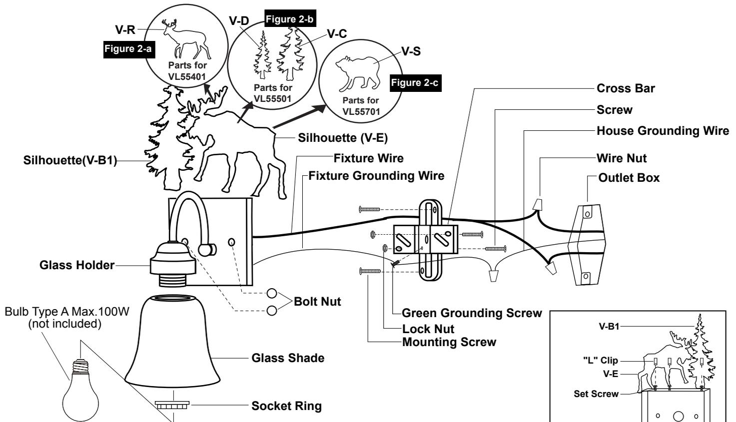
1. Thread two screws to the cross bar, and then secure with two lock nuts. Adjust the length of the screws if necessary.
